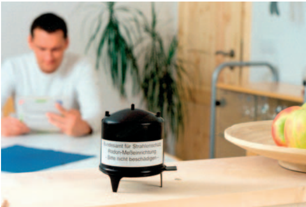
A radon detector that will measure radon concentrations for up to a year. It can also be placed on an open bookcase.
